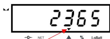
1. First count by hand a number of articles: 10, 20, 50, 100 or 200 pieces. The lighter the article, the more should be used for an accurate reference weighing.
